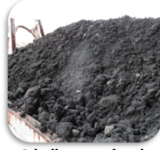
Grinding swarf and mill scale sludge
